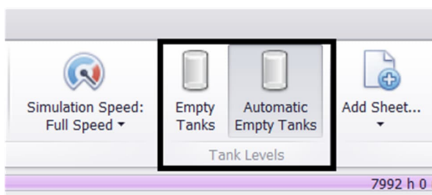
Figure 5: Tank levels toolbar section in Dynamic Settings. Automatic Empty Tanks is activated.
